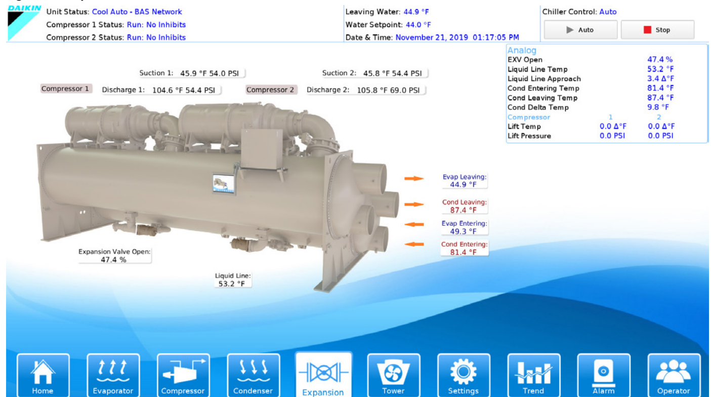
Figure 46: Expansion Valve Information
