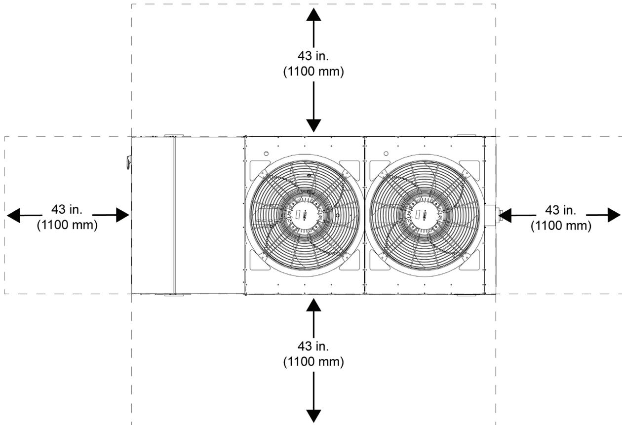
**Figure 6: Space Requirements - Installation Surrounded by Walls**
