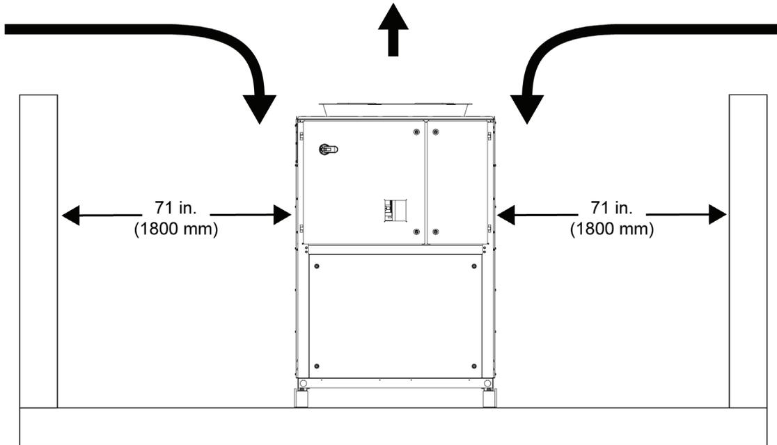
**Figure 7: Space Requirements - Installation with Wall Higher than Unit**
