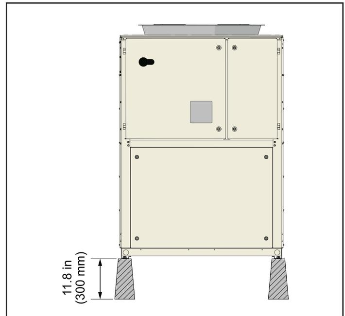
To install the anti-vibration supports, follow the instructions in the dimensional diagram supplied with the unit. The frame must be perfectly leveled during installation, if necessary by inserting shims under the anti-vibration supports.
