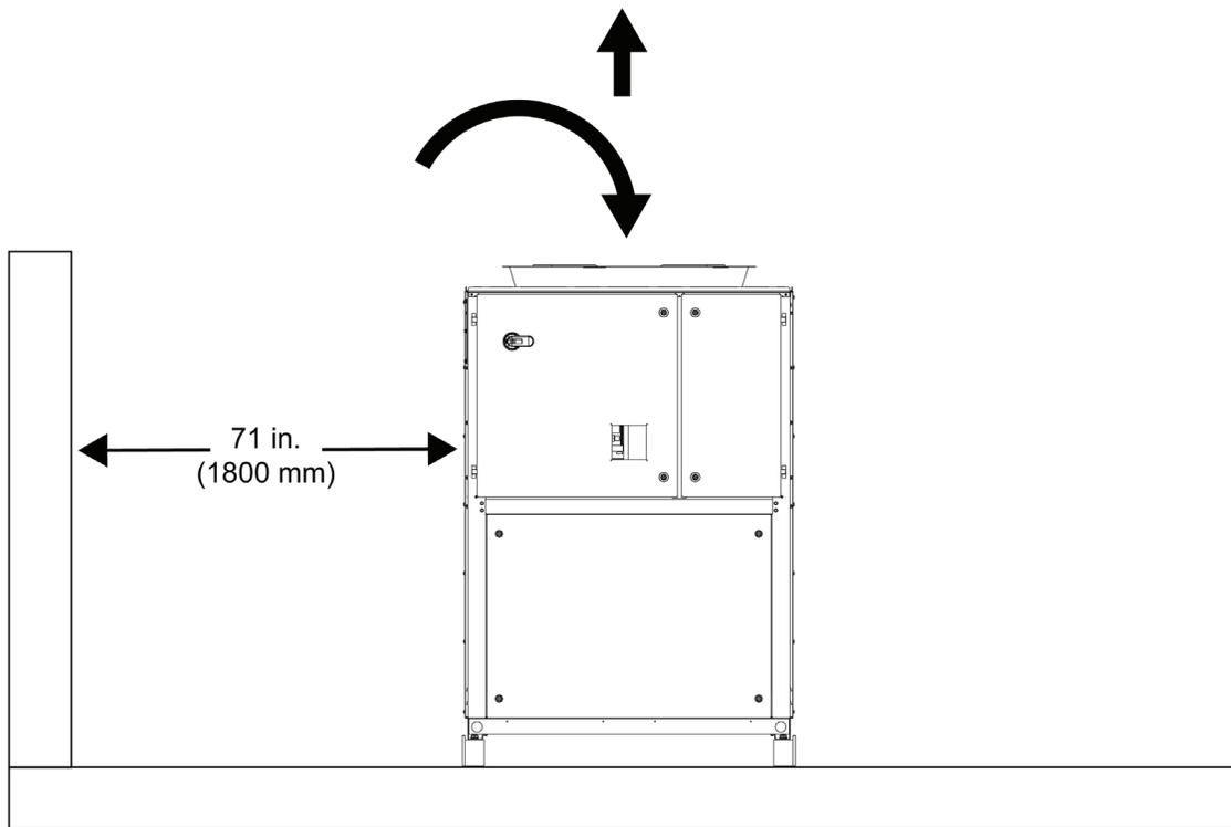
**Figure 8: Space Requirements - Minimum Distance Between Units**
