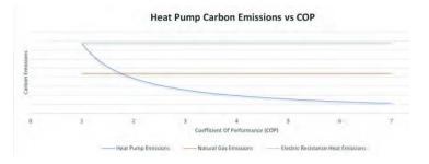
emissions tied to creating electricity) of the electrical grid. CO2 emissions of heating with natural gas are plotted in orange. In grey, we see the emissions of electric resistance heat. Comparing the two, we see that electric resistance heat has higher CO2 emissions than direct natural gas heating due to the fossil fuels used to generate the electricity.
