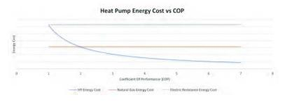
By increasing the overall efficiency of the heat pump and improving the low-ambient performance, inverters improve the average efficiency of the unit and make it more advantageous from an emissions perspective. Just as there is a crossover point for carbon emissions, the same is true if we map out energy costs, as shown in Figure 2. Depending on the location and corresponding cost of electricity and natural gas, as the heat pump COP improves so do the operating hours
