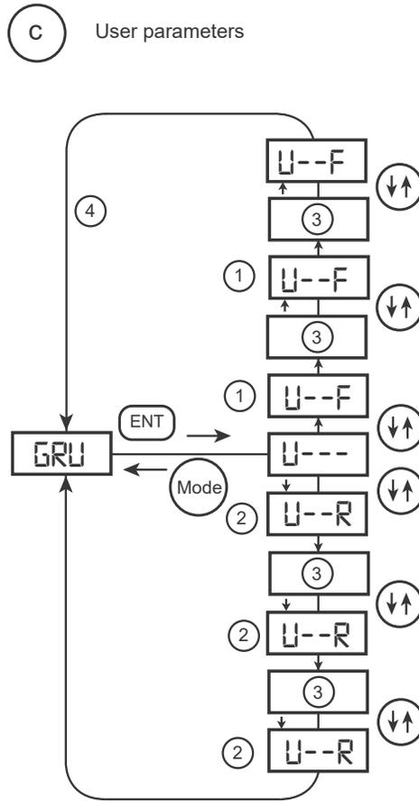
1. Pressing the UP key searches the parameter list starting with the first one changed.
