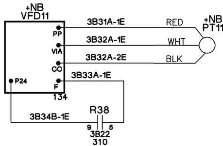
PT11 is a refrigerant pressure sensing transducer
