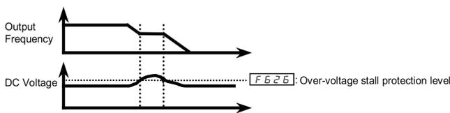
If **F 305** is set to 2 (quick deceleration), the drive controller will increase the voltage to the motor (over-excitation control) to increase the amount of energy consumed by the motor when the voltage reaches the overvoltage protection level. The motor can therefore be decelerated more quickly than with normal deceleration.
