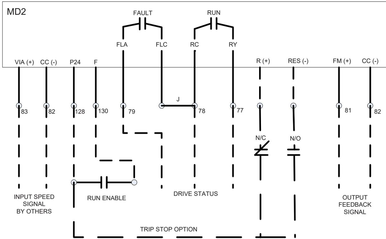
**NOTE:** Contacts and wire terminations are in the unit control panel. Terminal numbers designations are not applicable to Vision, Skyline, and Destiny units.
