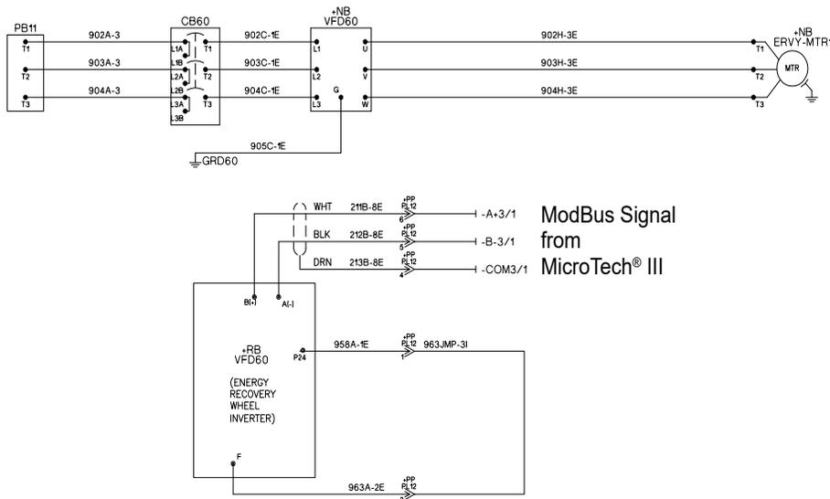
**NOTE:** Contacts and terminations are in the unit control panel.
