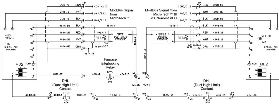
**NOTE:** Contacts and terminations are in the unit control panel.
