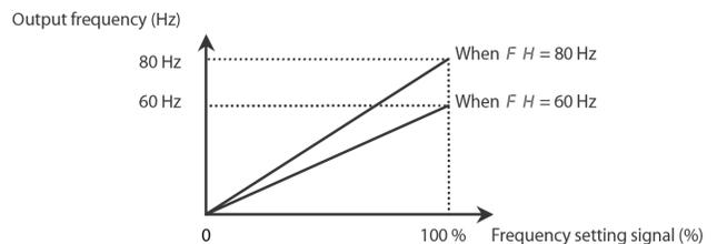
**NOTE:**  $F_H$  can not be adjusted during operation,  $\text{UL}$  value can not exceed  $F_H$  value.
