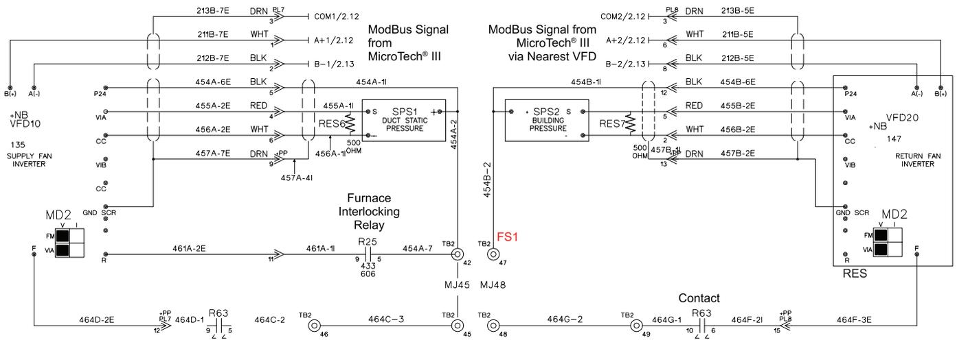
**Figure 32: Smoke Purge Wiring Diagram**
