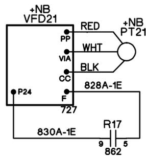
PT21 is a refrigerant pressure sensing transducer
