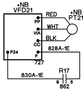
PT21 is a refrigerant pressure sensing transducer
