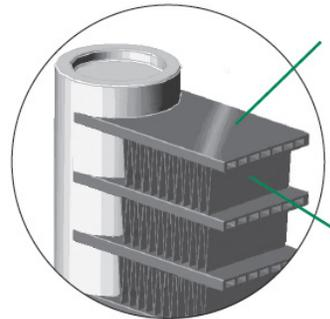
Flat aluminum tubes with many small flow channels increase fluid-to-tube heat transfer and reduce refrigerant charge requirements.
