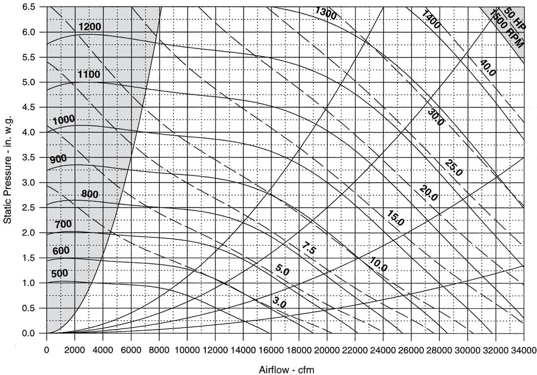
**NOTE:** Maximum allowable static pressure at fan bulkhead is 5.0 in. (i.e., supply duct ESP cannot exceed 5.0 in).
