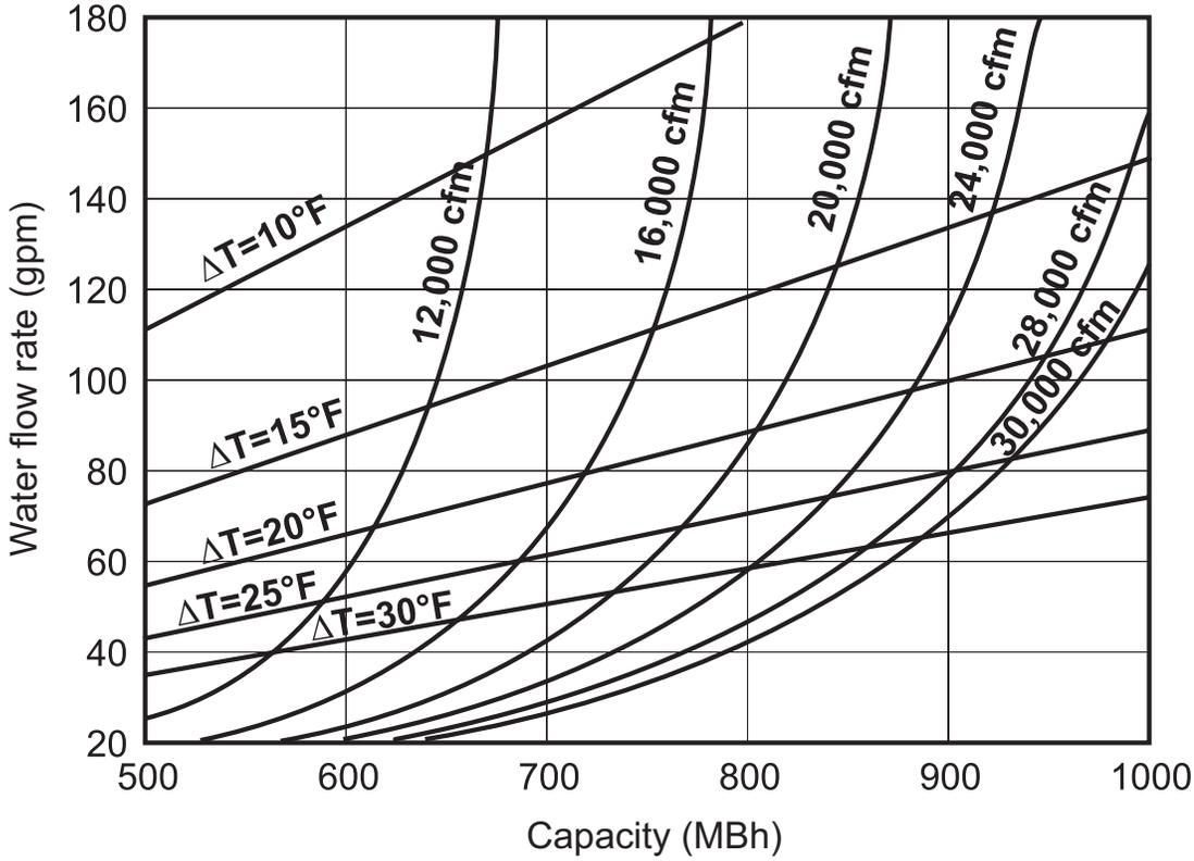
Figure 28: MPS 061-075 High Heat
