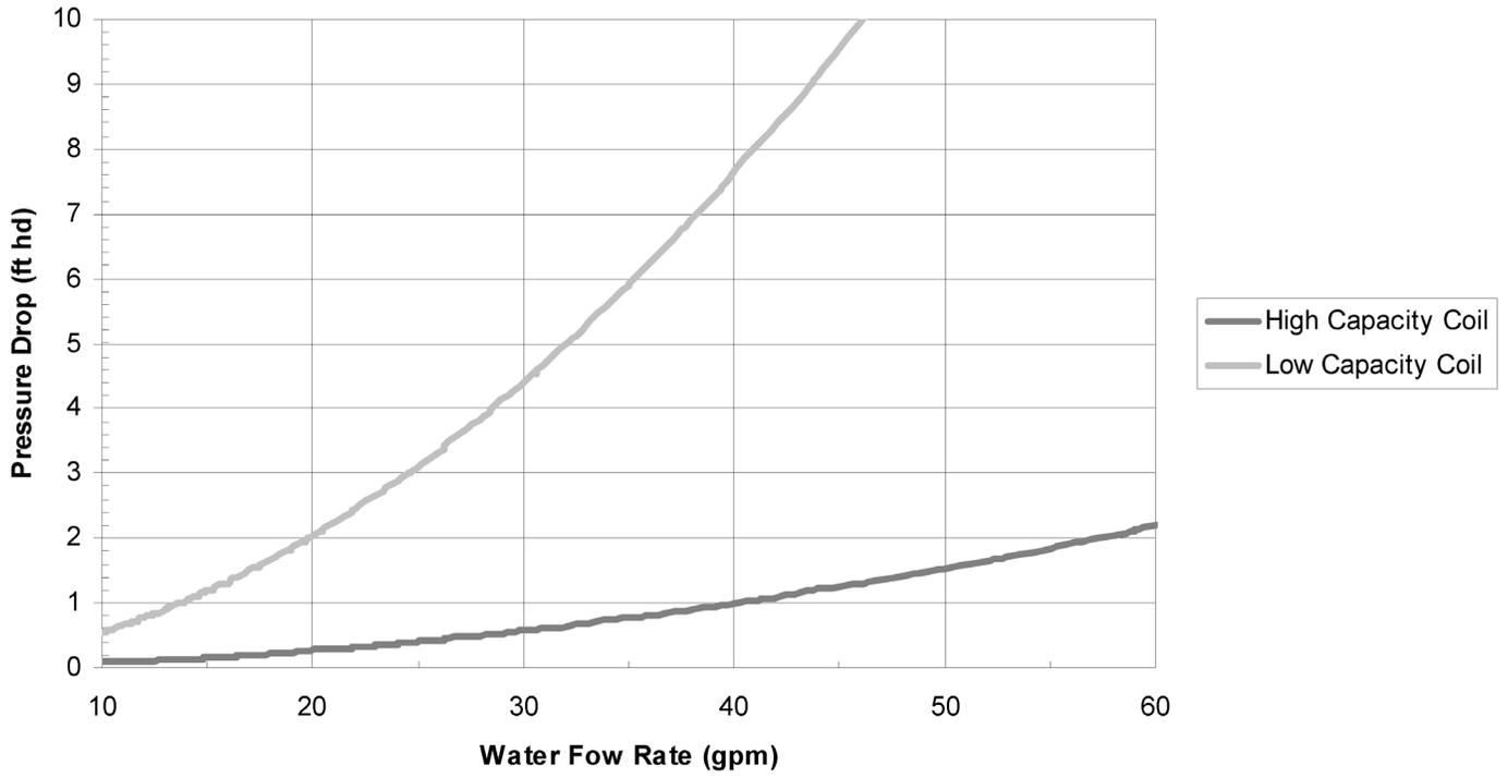
Figure 32: MPS 040–050 Pressure Drop
