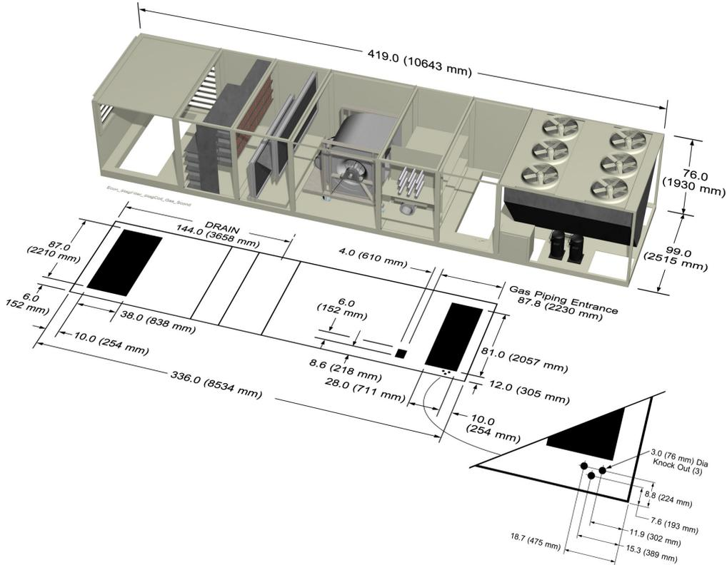
Figure 70: Shortest MPS 061 Cooling Only Unit
