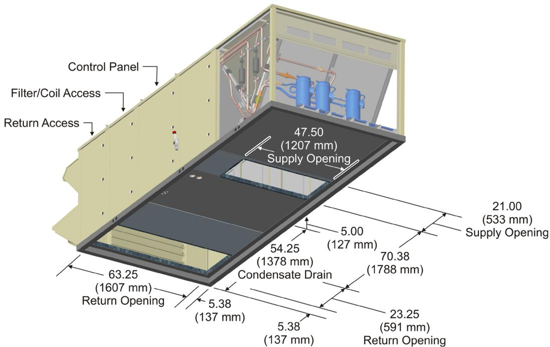
Figure 47: MPS 015-020 Cooling/Hot Water Heating Unit
