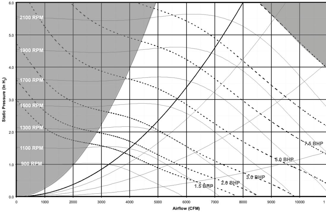
**Figure 35: 22-in. SWSI Airfoil Supply Fan**
