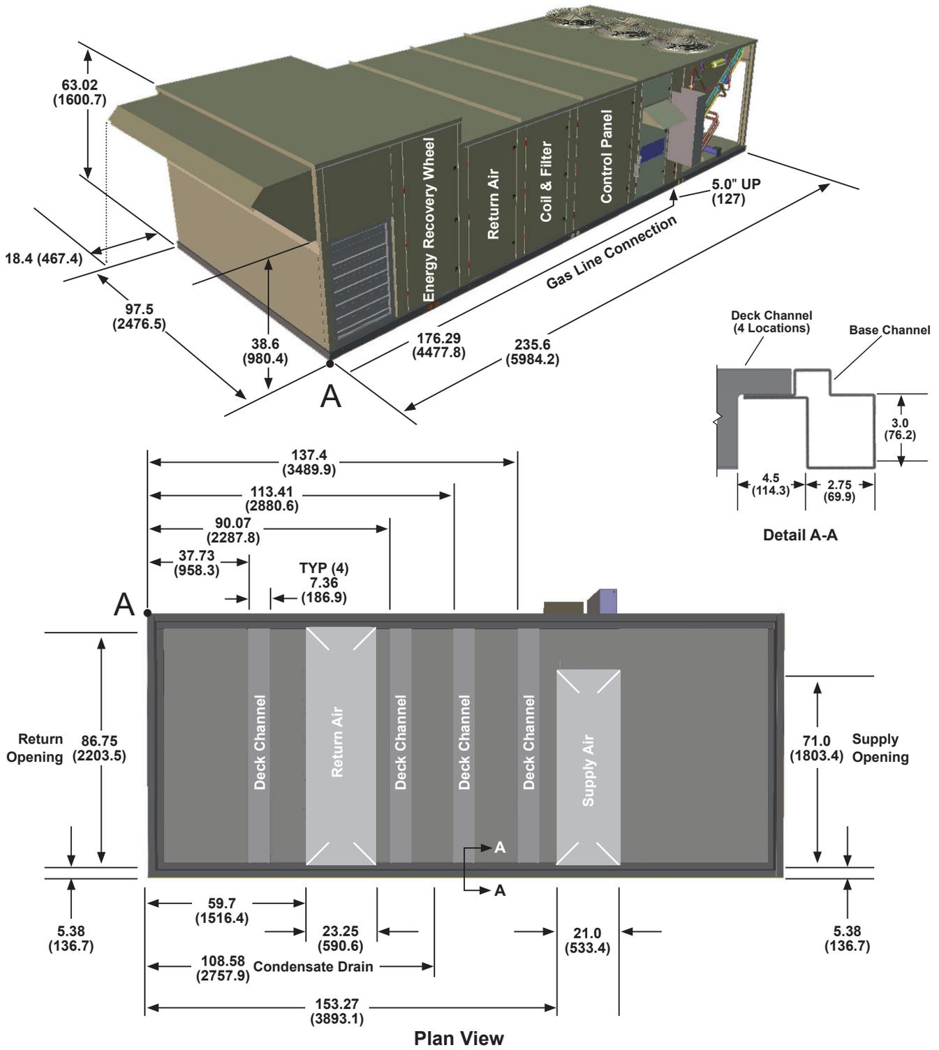
Figure 60: MPS 026–035 Gas Heat, Large Diameter Energy Recovery Wheel
