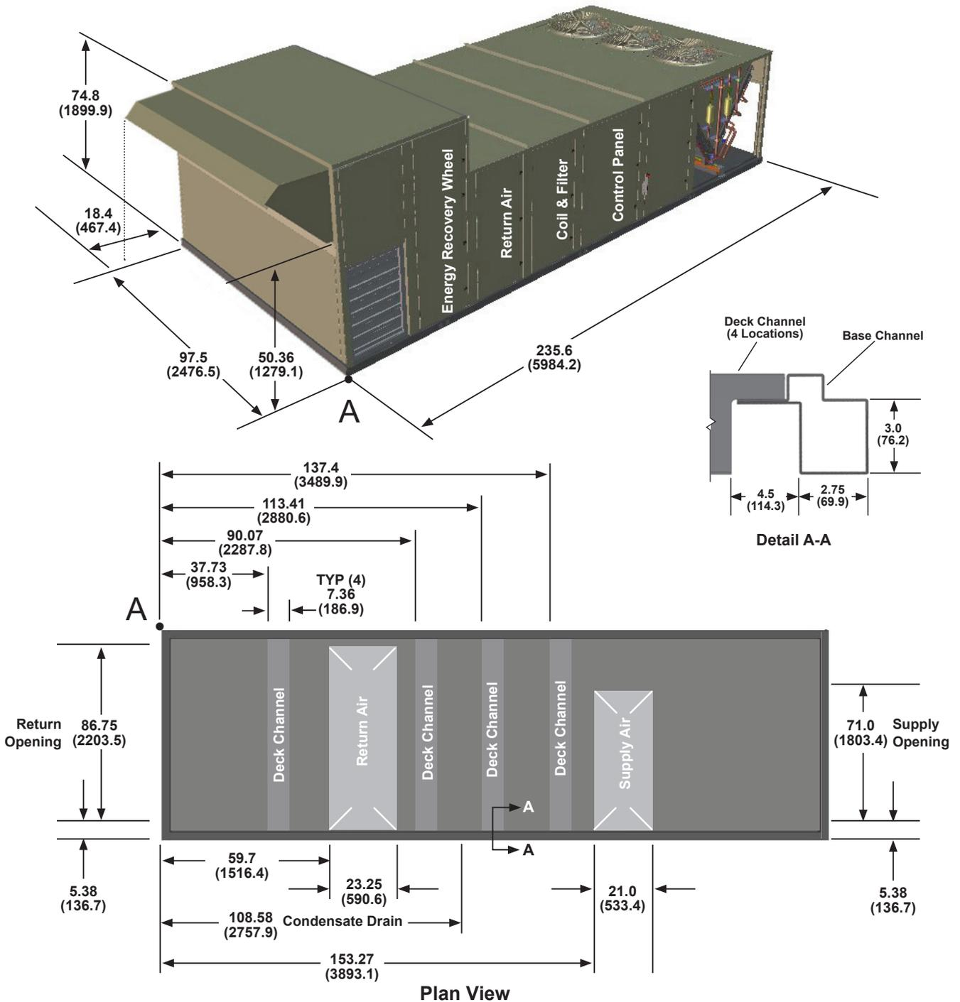
Figure 59: MPS 026–035 Gas Heat, Standard Diameter Energy Recovery Wheel
