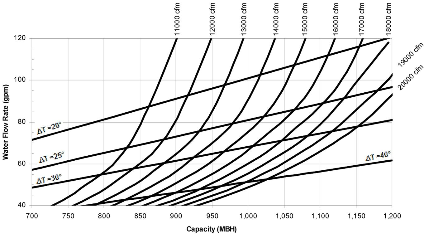
Figure 27: MPS 061-075 Standard Heat
