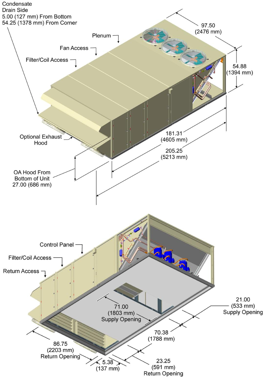
Figure 54: MPS 026–035 Cooling/Hot Water Heating Unit
