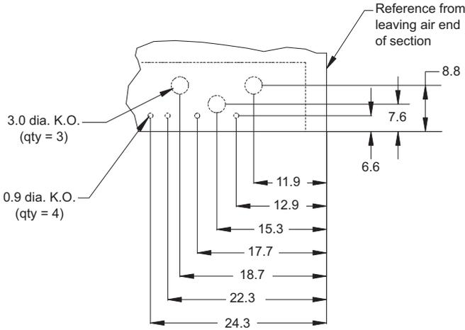
Figure 79: Main Control Panel/Discharge Plenum Knockout Detail
