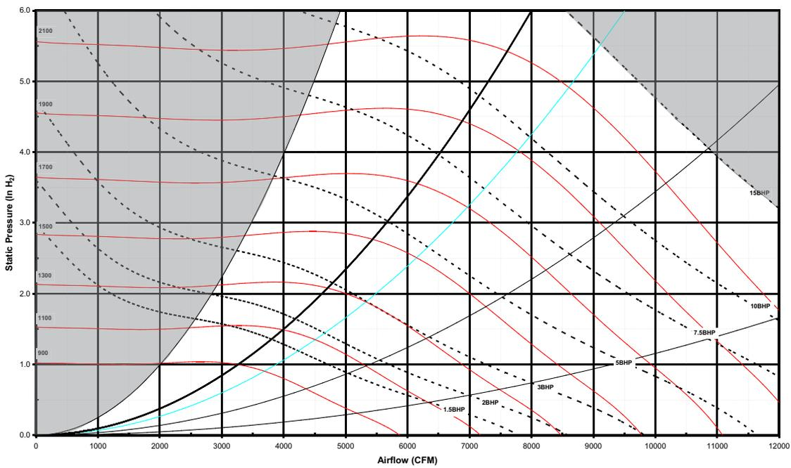
Figure 36: 24-in. SWSI Airfoil Supply Fan
