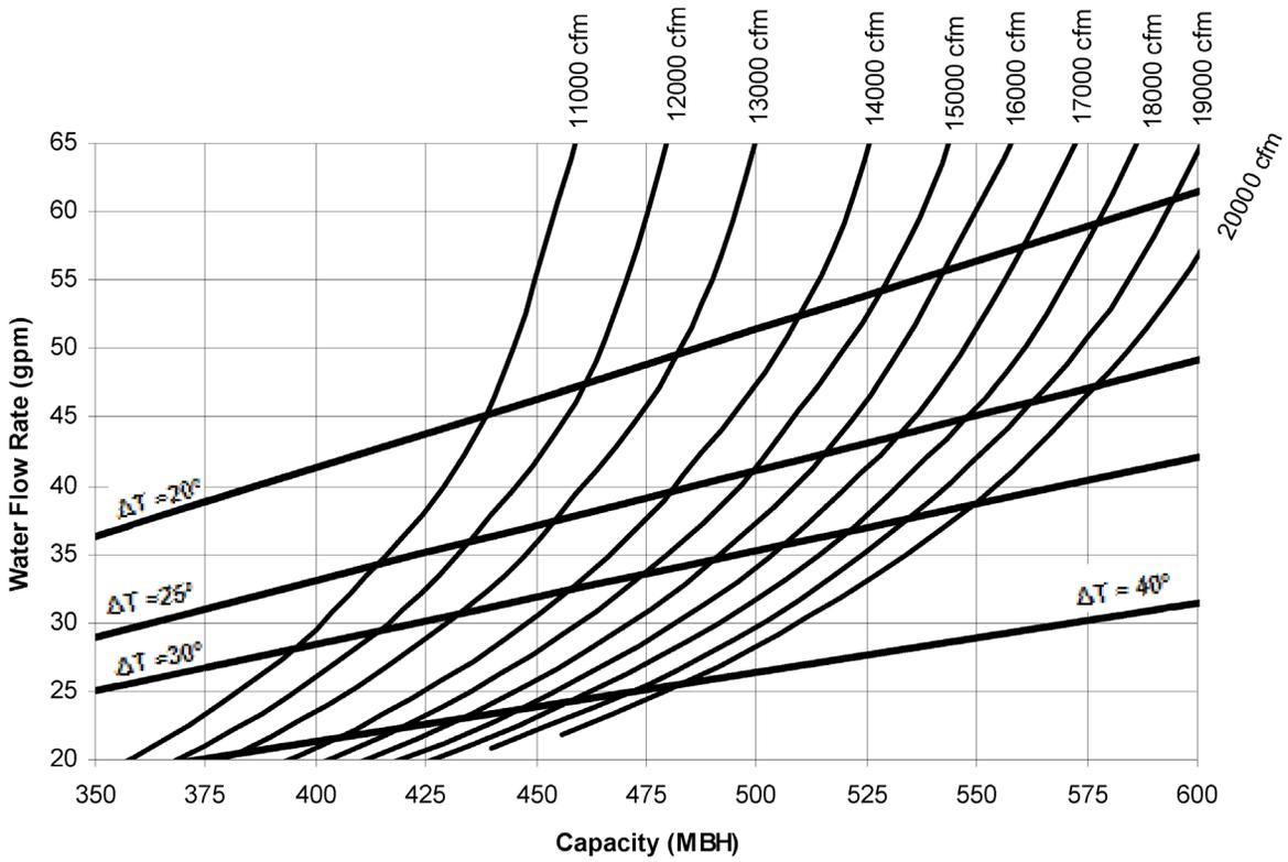
Figure 26: MPS 040–050 High Heat
