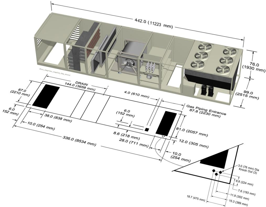
Figure 72: Shortest MPS 070–075 Cooling Only Unit
