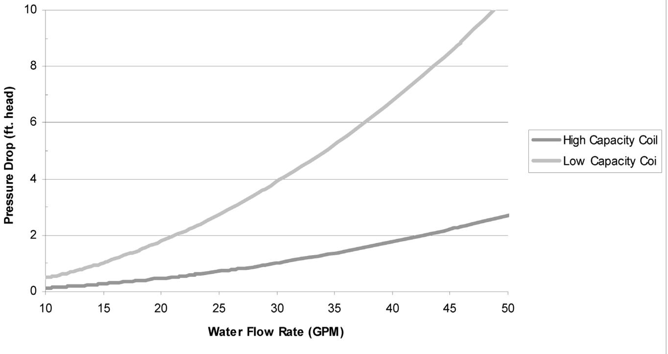
Figure 30: MPS 020 Pressure Drop
