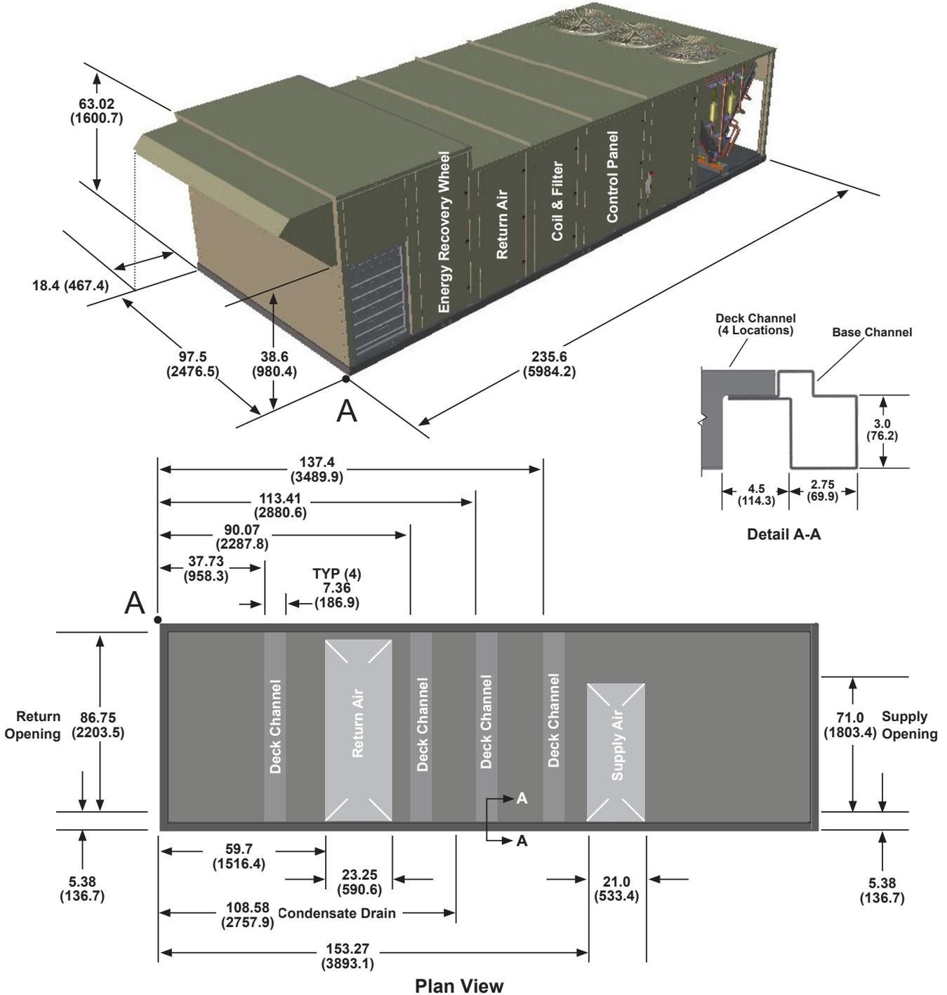
Figure 58: MPS 026–035 Cooling Only, Large Diameter Energy Recovery Wheel
