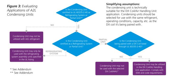
Condensing units are also tested as a partial unit in accordance with UL 60335-2-40. This allows operation with other 60335-2-40 partial units, including partial unit listed DX coils and air handling units, assuming the equipment is technically suitable and utilizes the same refrigerant (Figure 3).
