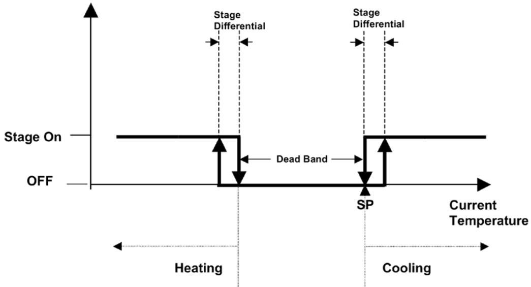
Figure 18: Cooling and Heating Control, Auto Changeover, Dead band Option = 1
