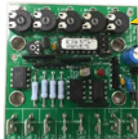
Rotate dial(s) clockwise to increase max CFM or counter clockwise to decrease. Call 1, 2 & 3 are used with 3 spd fan thermostat. (Call 4 not used)
