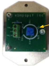
Rotate dial clockwise to increase max CFM or counter clockwise to decrease. (Used with 0-10VDC fan speed signal)
