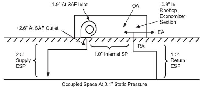
Figure 33 illustrates how adding a return fan corrects these problems. The return fan is responsible for return system ESP and maintains a slightly positive pressure in the economizer section (about +0.1" in Figure 33) to allow for exhaust air control and a more suitable outside air intake pressure.
