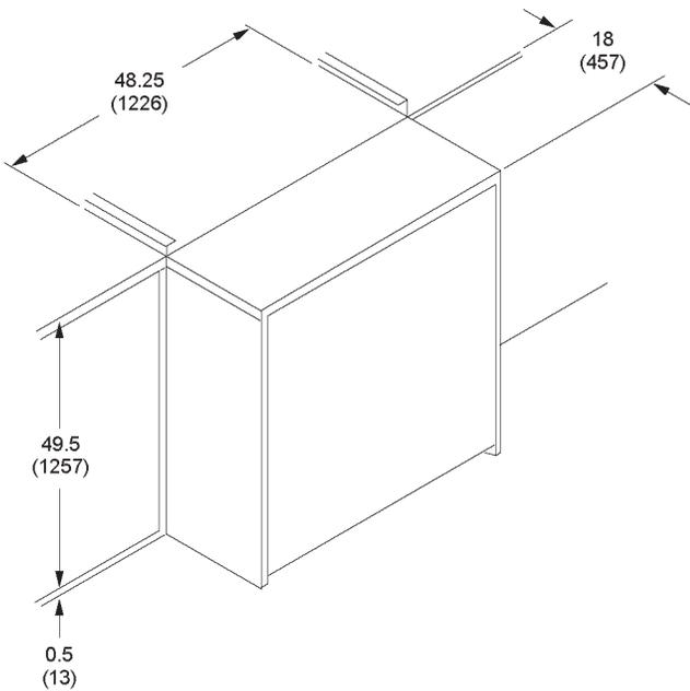
Note: Vestibule required for 48" long coil with piping entering within the curb and recommended for piping entering the side of the unit.
