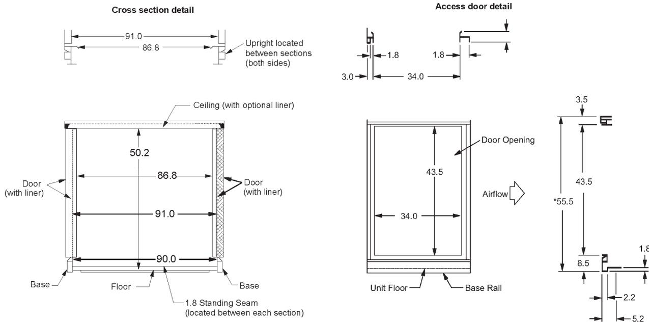
Figure 98: Field-installed coil piping vestibule detail—RDS 800C and RDS 802C
