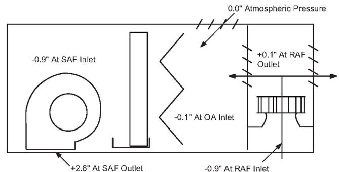
Exhaust fans are very different than return fans and cannot maintain proper building pressure and ventilation control as return ESP increases.
