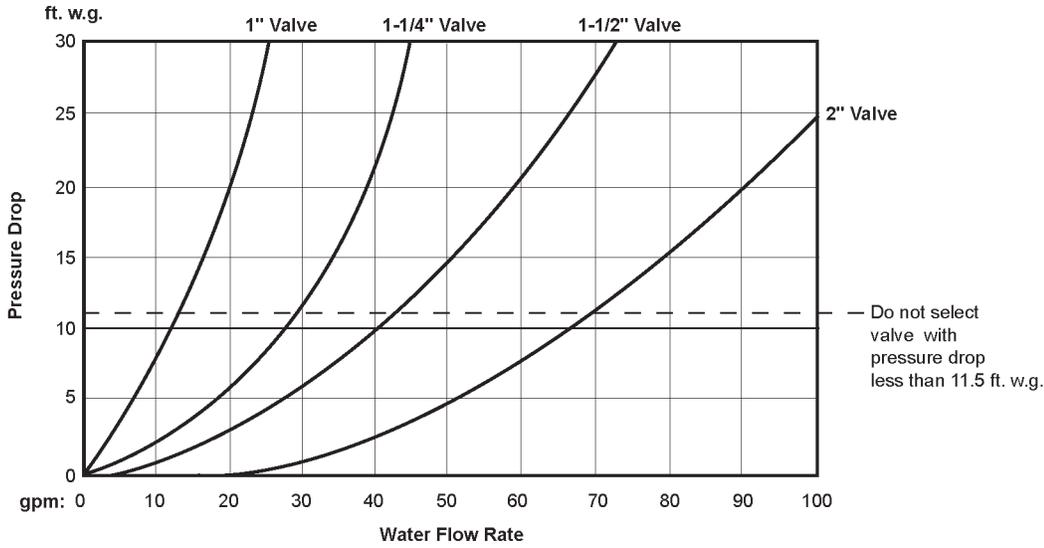
Figure 40: Unit hot water valve and piping pressure drop
