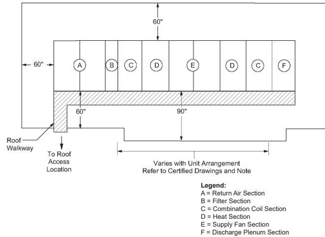
Figure 120: Service clearances—RAH unit with housed DWDI supply fan
