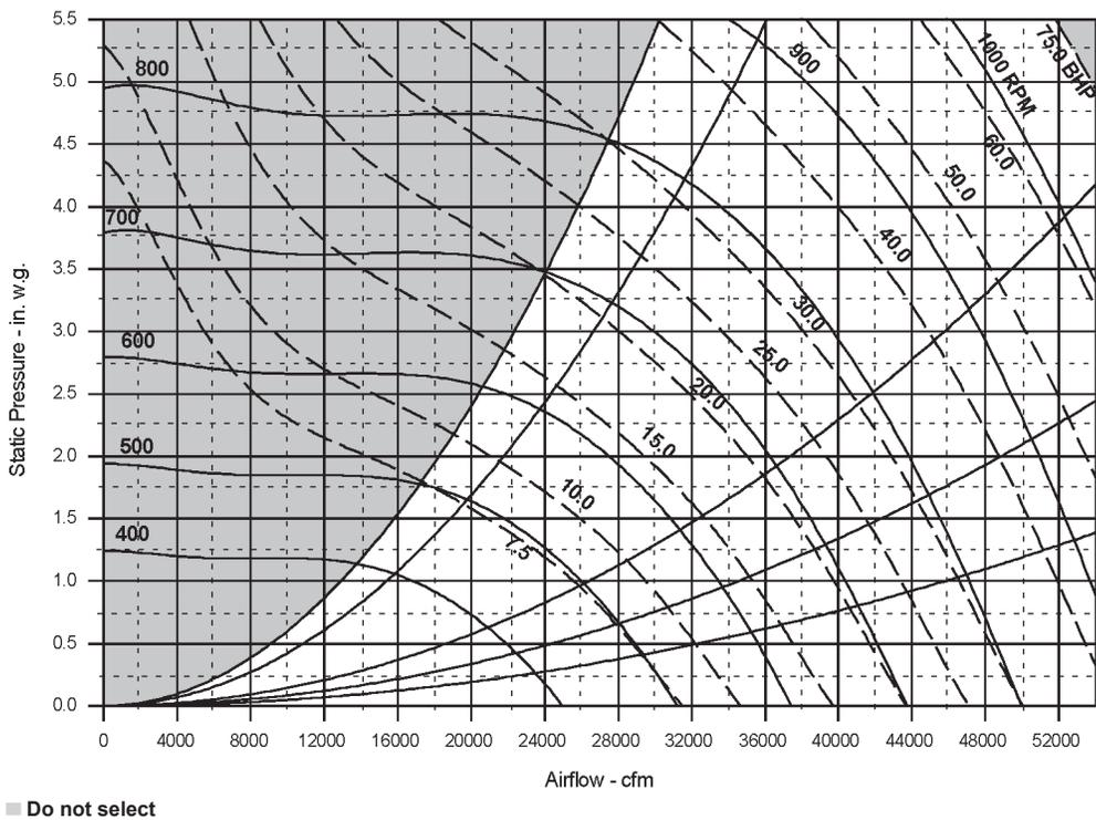
**NOTE:** Maximum allowable static pressure at fan bulkhead is 5.0 in (i.e., ESP plus blow-through component pressure drops cannot exceed 5.0 in).
