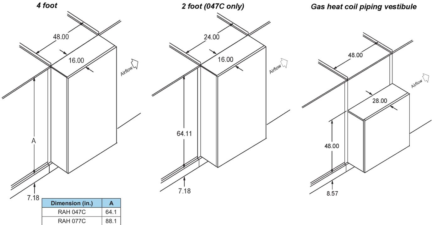
Blank Access and Drain Pan Only Section Details—RAH 047C and RAH 077C
