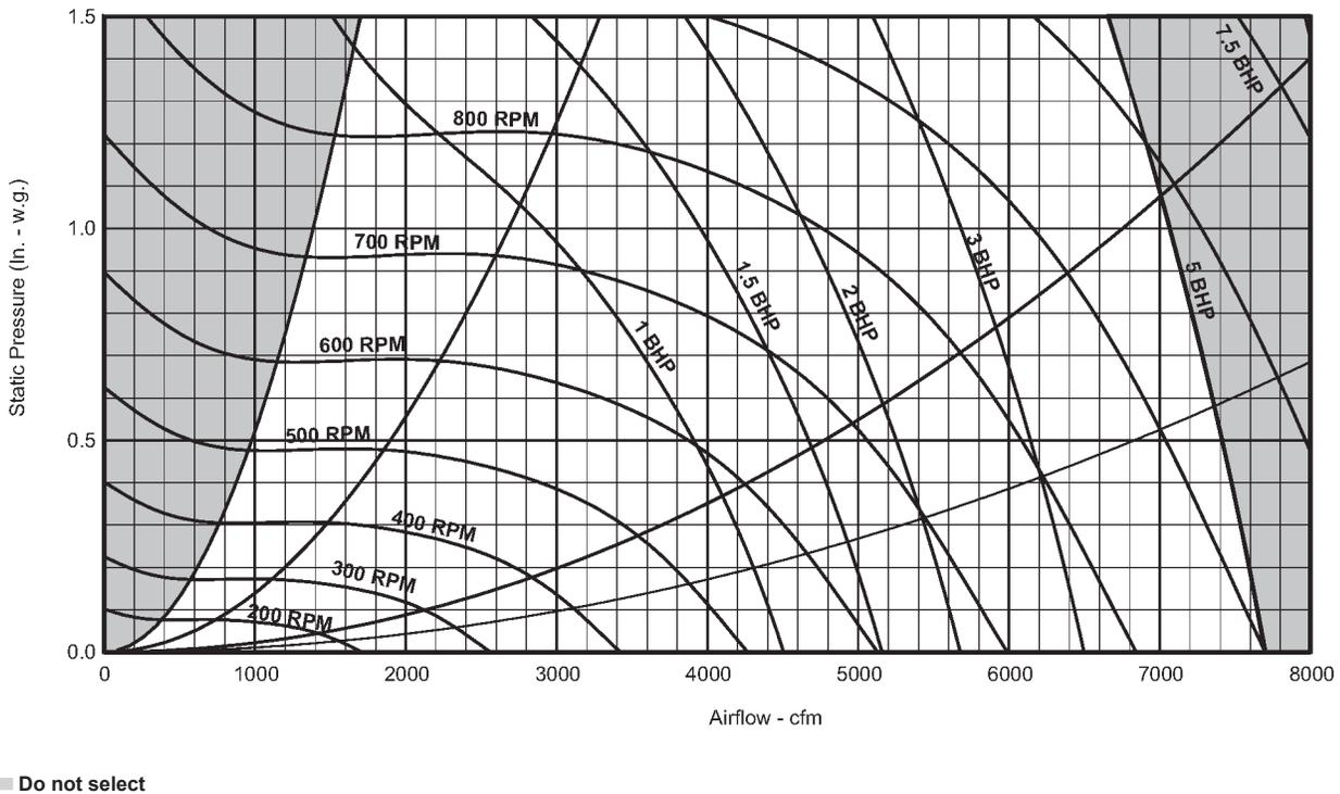
Figure 73: RDS 708B 16" airfoil fan without vanes
