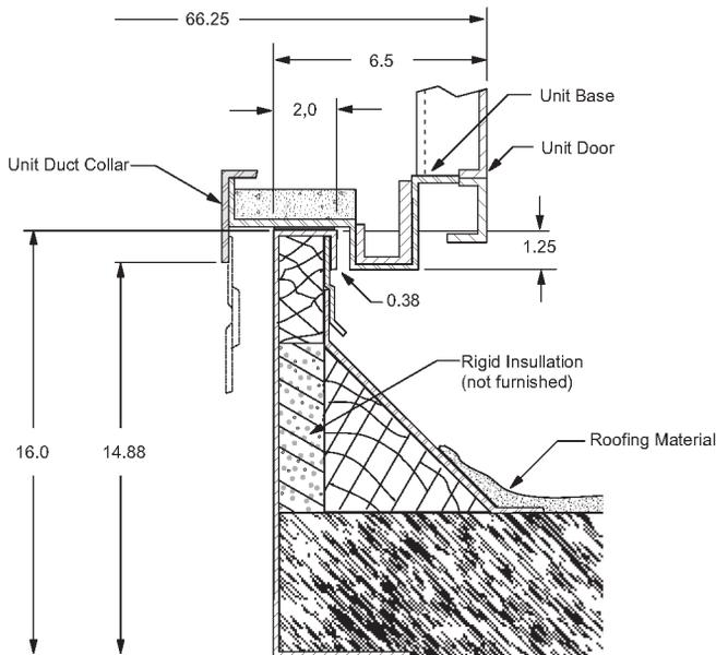
Figure 88: Curb cross section B-B
