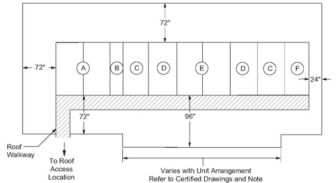
Note: Sections with heating and/or cooling coils or DWDI supply fan must have 98" service clearance on control box side.
