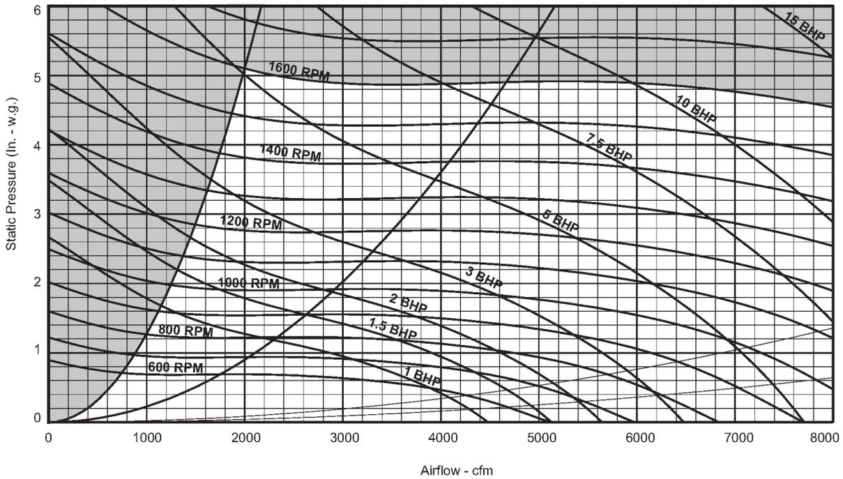
Figure 50: RDS 708B supply fan, 16" airfoil fan without vanes
