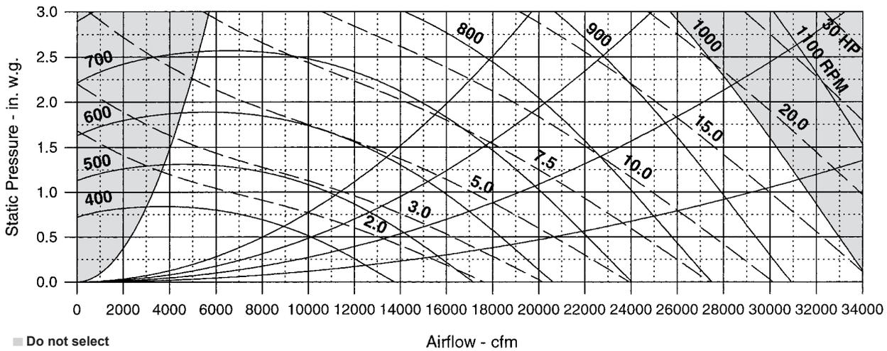
Figure 79: RAH 077C SWSI fan, 44" airfoil
