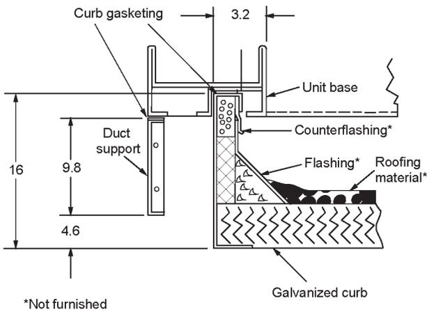
Figure 96: Curb cross section B-B
