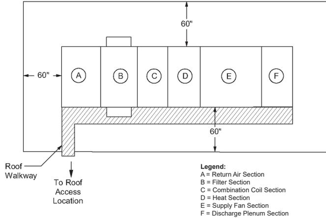
Figure 119: Service clearances—RAH unit with SWSI plenum supply fan
