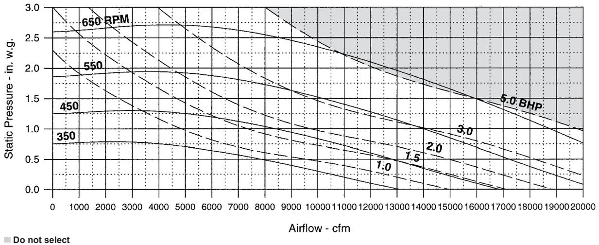
Figure 78: RAH 047C, SWSI fan, 40" airfoil
