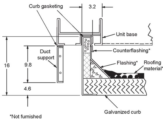
Figure 114: Curb cross section B-B
