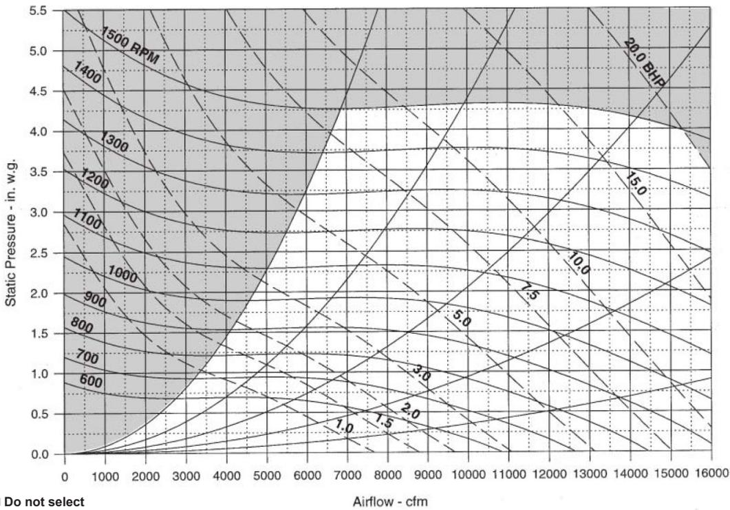
Figure 54: RDS 800C supply fan, 20" airfoil
