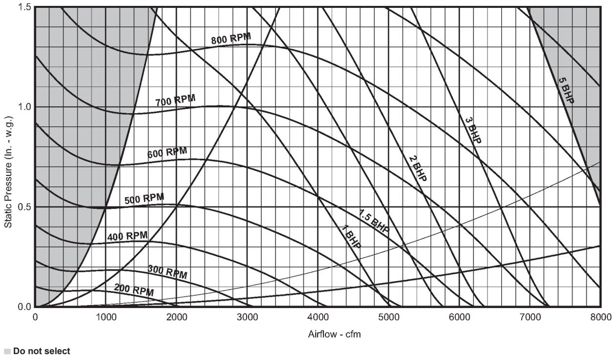
Figure 72: RDS 708B 15"×15" forward curved return fan with vanes
