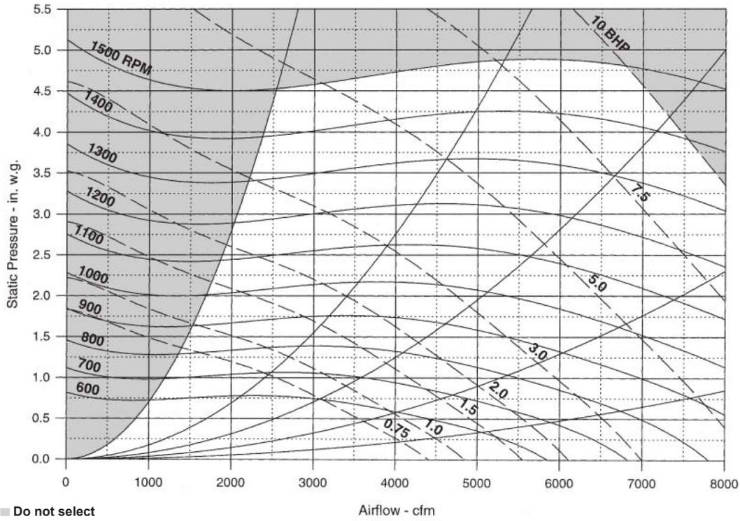
Figure 53: RDS 800C supply fan, (2) 15"×15" forward curved
