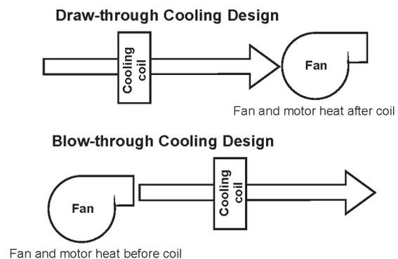
Figure 36: Blow-through vs. draw-through performance
