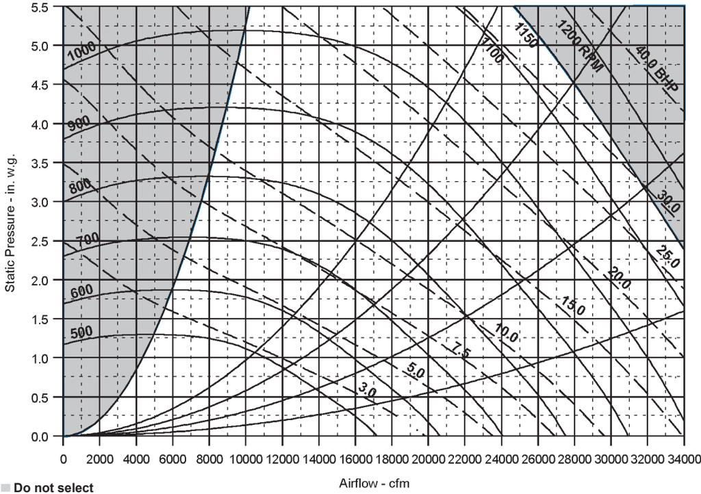
**NOTE:** Maximum allowable static pressure at fan bulkhead is 5.0 in (i.e., ESP plus blow-through component pressure drops cannot exceed 5.0 in).
