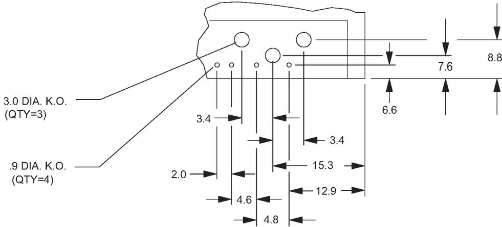
Note: 0.9 diameter and 3.0 diameter knockouts are electrical entrance locations on the unit only.
