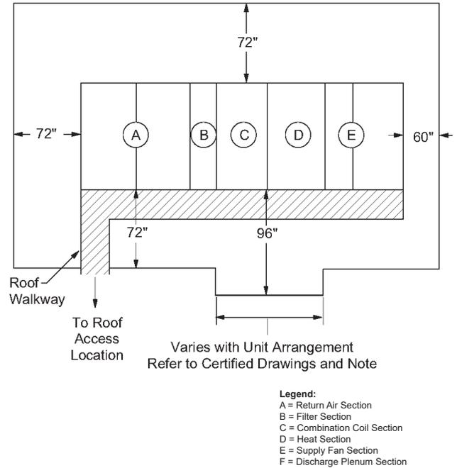
Figure 118: Service clearances—RDS 800C and 802C
