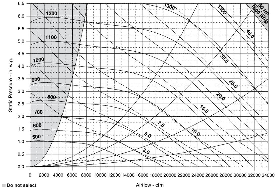
**NOTE:** Maximum allowable static pressure at fan bulkhead is 5.0 in (i.e., ESP plus blow-through component pressure drops cannot exceed 5.0 in).
