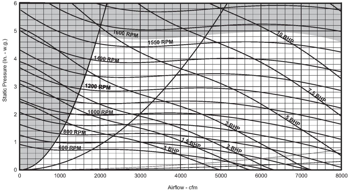
Figure 49: RDS 708B supply fan, 15"×15" forward curved fan with vanes
