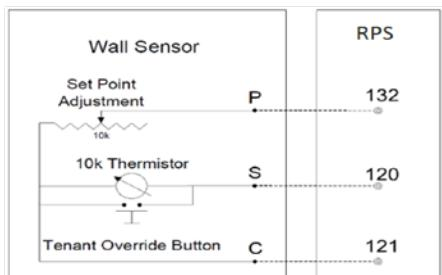
Note: Shield wire is to be grounded at the RTU chassis only.
