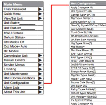
5. Once all the values under the Unit Configuration menu are confirmed, set the Apply Changes parameter to Yes and press the enter button.
