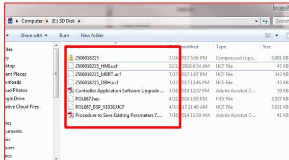
6. This completes preparing the SD card for the download process and should be now taken to the Microtech controller.
