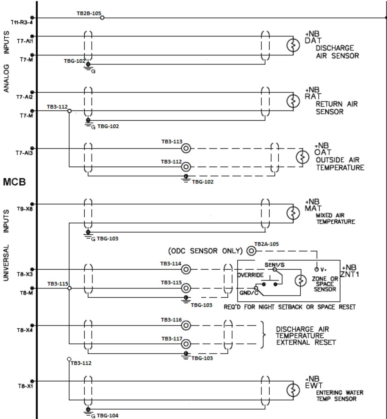
Figure 14: Sensor Wiring Diagram
