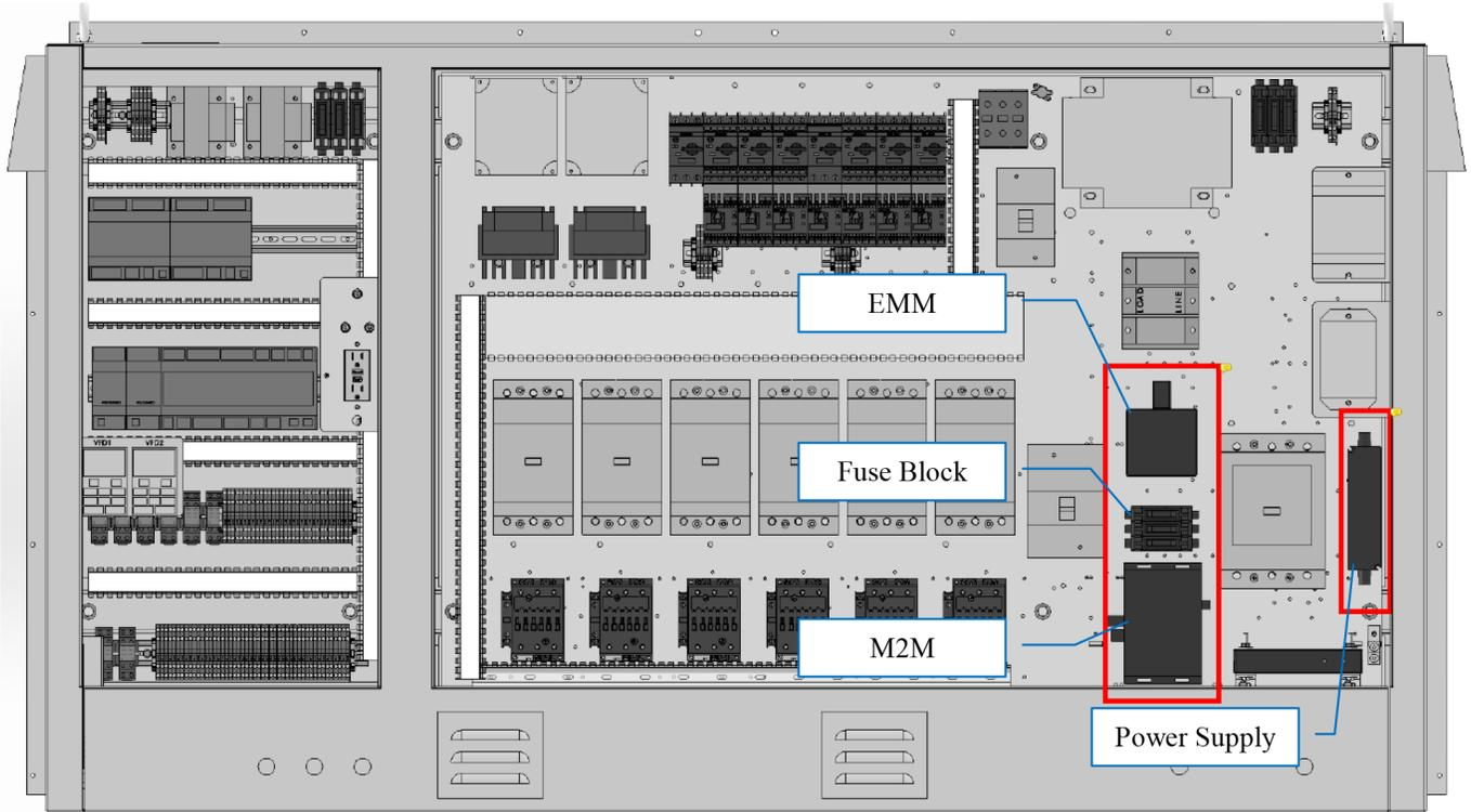
Figure 2: Typical MicroTech Control Panel Layout - 045C - 135C, 047C and 077C
