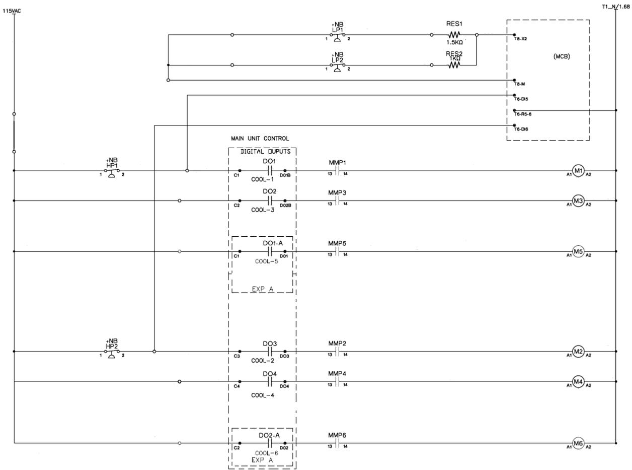
Figure 22: MicroTech I 6-Compressor/6-StageFigure
