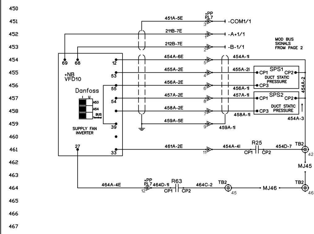
Figure 48: Schneider VFD Wiring
