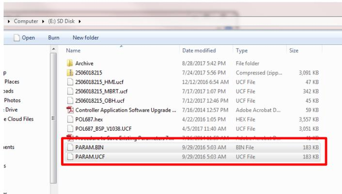
8. If the files are not saving to the existing SD card then check the SD card lock or try a different SD card
