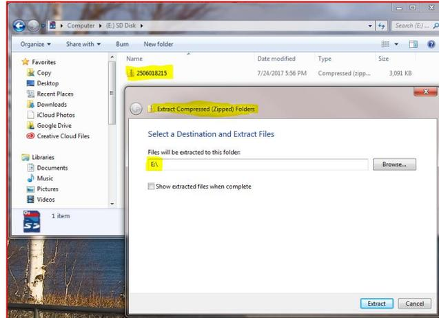
5. Once all the files are extracted there will be a total of 8-9 files appearing on the SD card. Total files counts can change with new software revisions. The list below show critical files needed for a software download.
