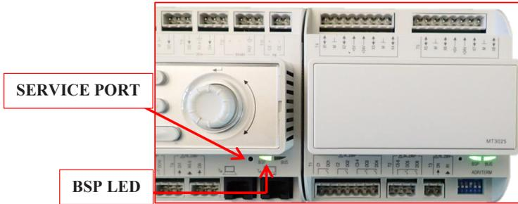
4. While holding the service button depressed, apply power to the controller.
