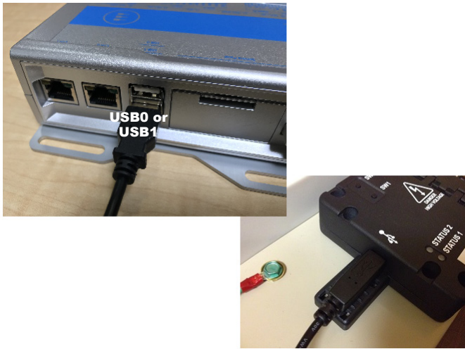
Figure 81: USB Connections (Generation 2 Gateway)
