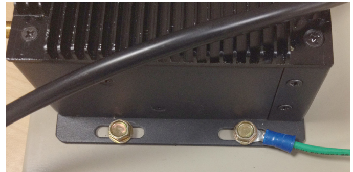
Figure 12: Installation of Grounding Ring to M2M Gateway (Shown with Generation 1 Gateway)
