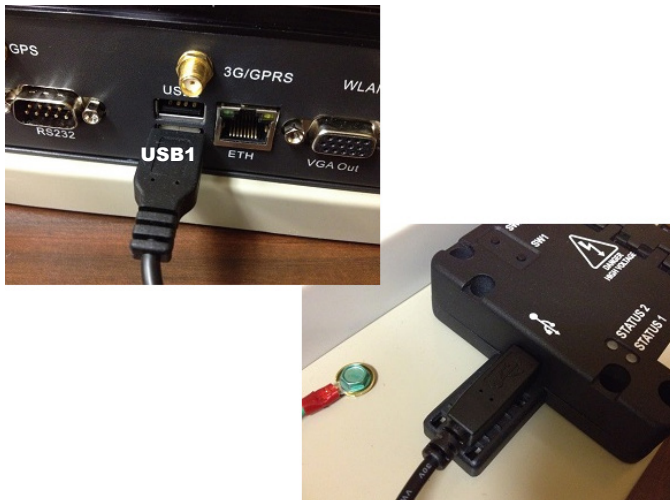
Figure 23: USB Connections (Generation 1 Gateway)
