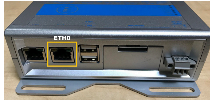
Figure 59: LAN Connection (Generation 2 Gateway)
