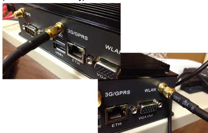
Figure 57: Cellular and Wi-Fi Connections (Generation 2 Gateway)
