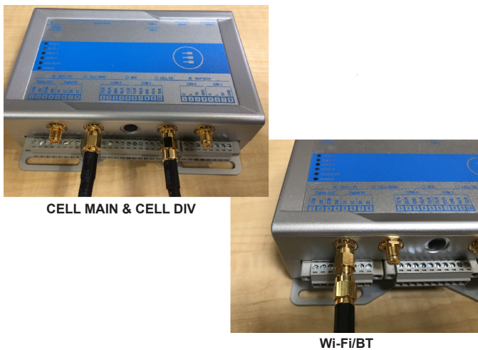
Figure 98: Cellular and Wi-Fi Connections (Generation 2 Gateway)
