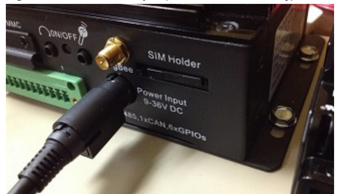
Figure 30: M2M Power Input (Generation 2 Gateway)
