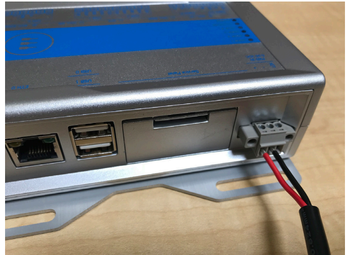
Figure 83: M2M Gateway Power Input (Generation 2 Gateway)
