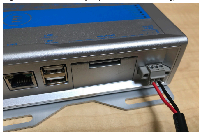
Figure 30: M2M Power Input (Generation 2 Gateway)
