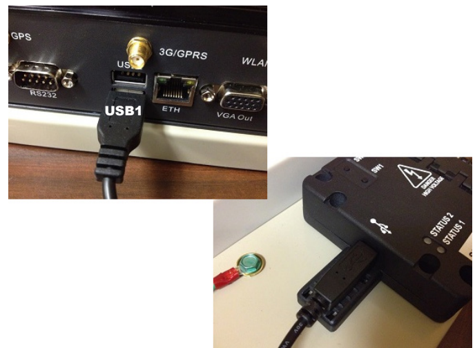
Figure 80: USB Connections (Generation 1 Gateway)
