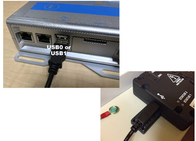
Figure 24: USB Connections (Generation 2 Gateway)
