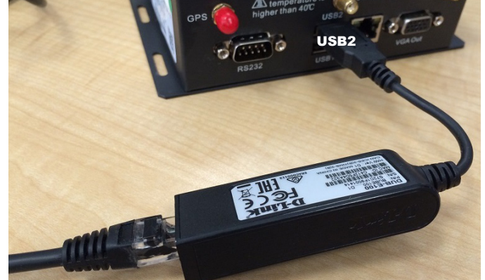
Figure 58: LAN Connection (Generation 1 Gateway)
