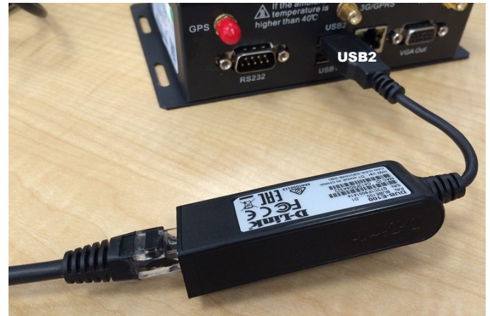
Figure 100: LAN Connection (Generation 2 Gateway)
