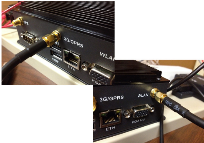
Figure 98: Cellular and Wi-Fi Connections (Generation 2 Gateway)
