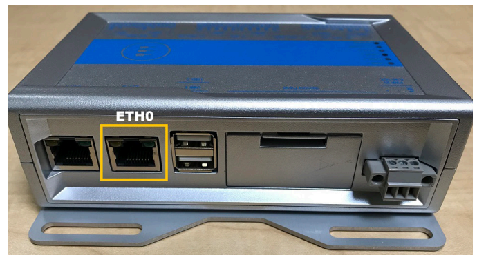
Figure 100: LAN Connection (Generation 2 Gateway)
