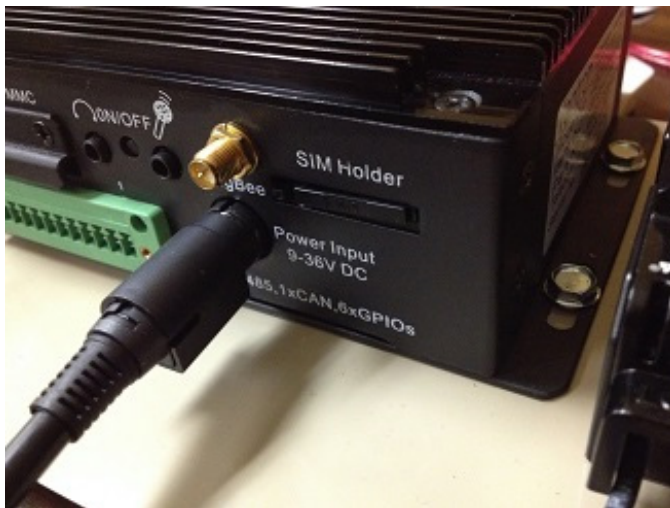
Figure 82: M2M Gateway Power Input (Generation 1 Gateway)
