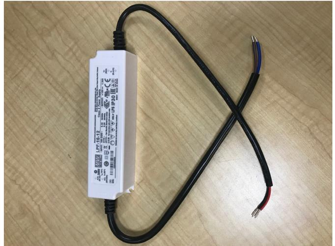
**Figure 16: Generation 2 Gateway Power Input (Generation 2 Gateway)**
