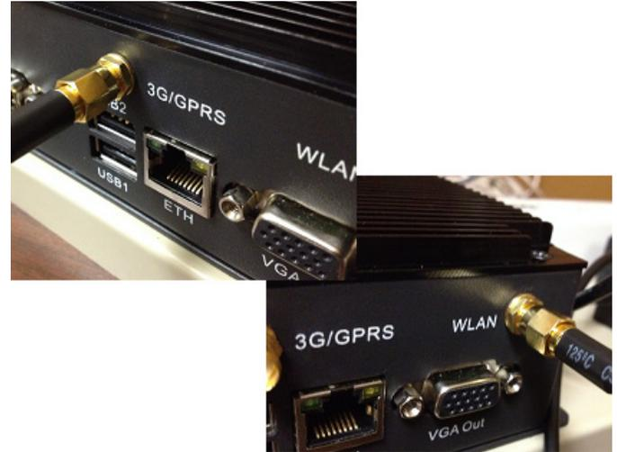
If the application is LAN, unplug the USB-to-Ethernet adapter (Figure 8) from the "USB2" port of the Generation 1 Gateway.
