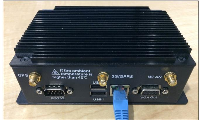
Figure 11: Generation 2 Gateway Connection
