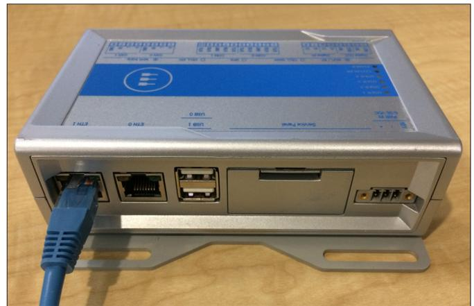
Figure 8: Connect Gateway Power Supply
