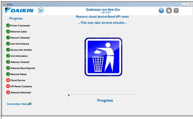
**Figure 20: Resetting the Cloud API**
