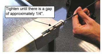
**STEP 4:** Once all four corner latches have been tightened within 1/4" of the leg extension coupling, complete the installation by tightening each corner until the latch and leg extension coupling meet. This is illustrated in Figure 25.
