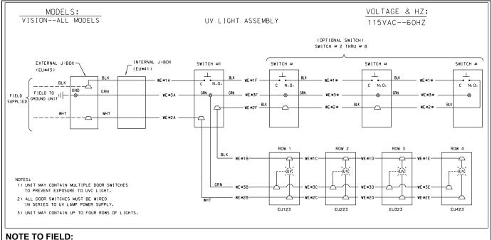
Switches are shown with the access panels in the open position. Lights are on when the access panels are closed and off when the access panels are open.
