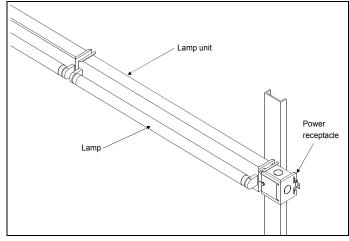
2. Unplug the power receptacle from the row of lamps by pulling it apart from the lamp unit. Then slide the receptacle off the rail. See Figure 3.
